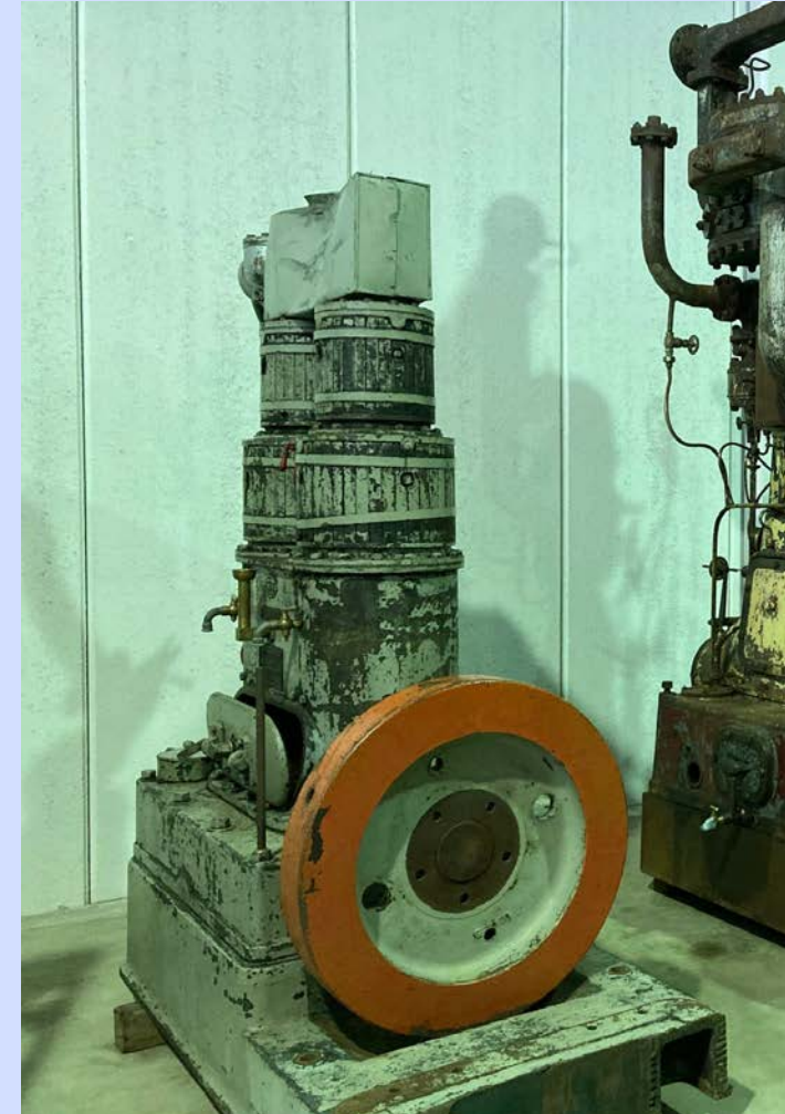
Twin cylinder Willans & Robinson vertical engine L-R before and after asbestos removal and encapsulation work, NMA Storage Facility, 8 McEacharn Place, Mitchell ACT AUSTRALIA, Image: Pippa Thorogood McLennan, 2025
